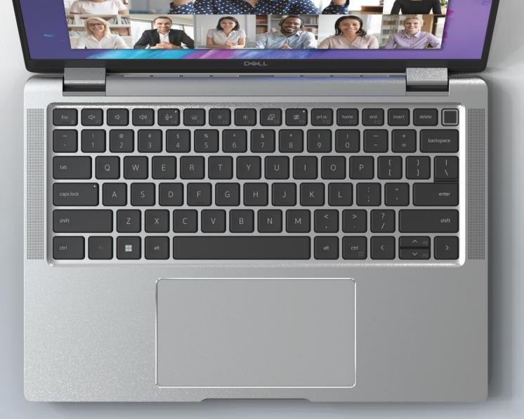
High-quality top and bottom firing speakers located on the side of the keyboard and below the front edge, deliver clear audio for when users are on conference calls.
