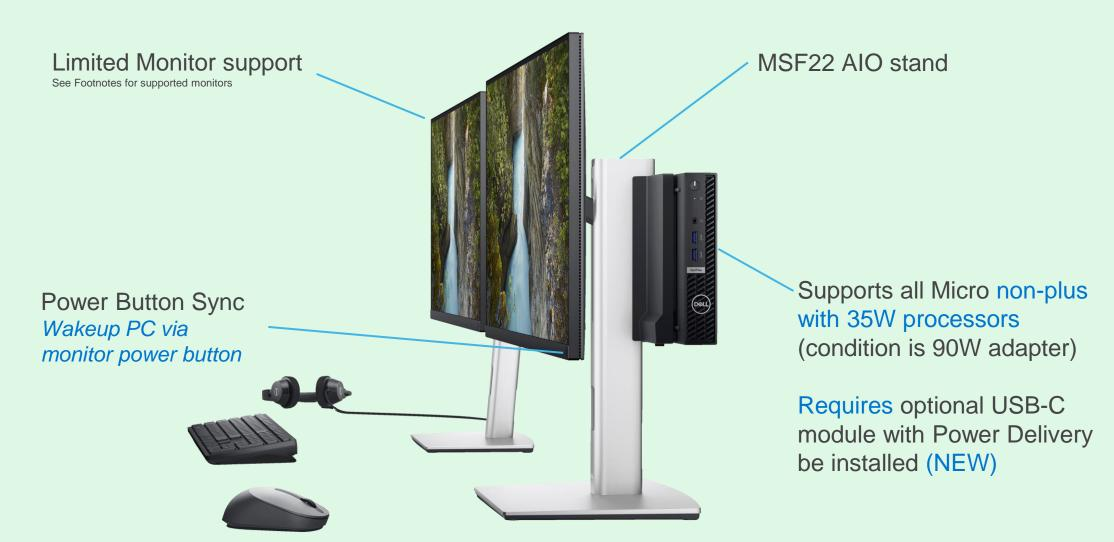
\*OptiPlex Micro Plus not supported due to higher power requirement (up to 180W)
